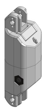
Place **1 x M10 spring** through the shown spot in previous assembly from step 3c.
