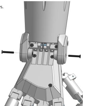
In the hand assembly, we have attached a tension spring to the hand. Now, we attach the other end of the tension spring in the shown spot on the forearm by pushing the rod till the end.
