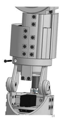
Guide the tubes from the assembly inside the channels in the shoulder as shown.
